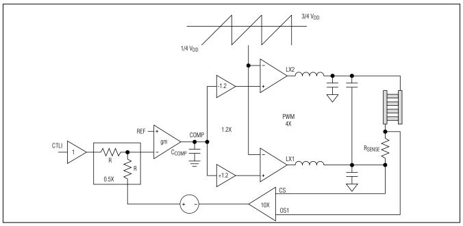
Figure 3. Functional Diagram of the Current-Control Loop
