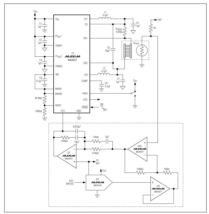
Figure 1. MAX8521 Typical Application Circuit
